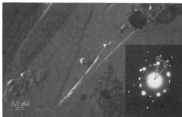
Figure 8. Twin crystal morphology with an angle of 25^\circ between two a -axes observed in TEM and ED.
